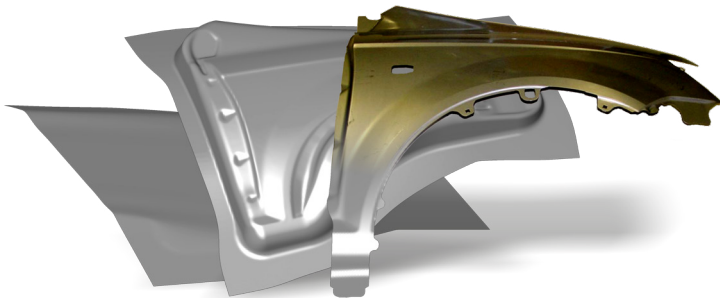
Stampack Trim Optimizer saves costly laser-cut prototypes and thus also valuable trial and development time.
