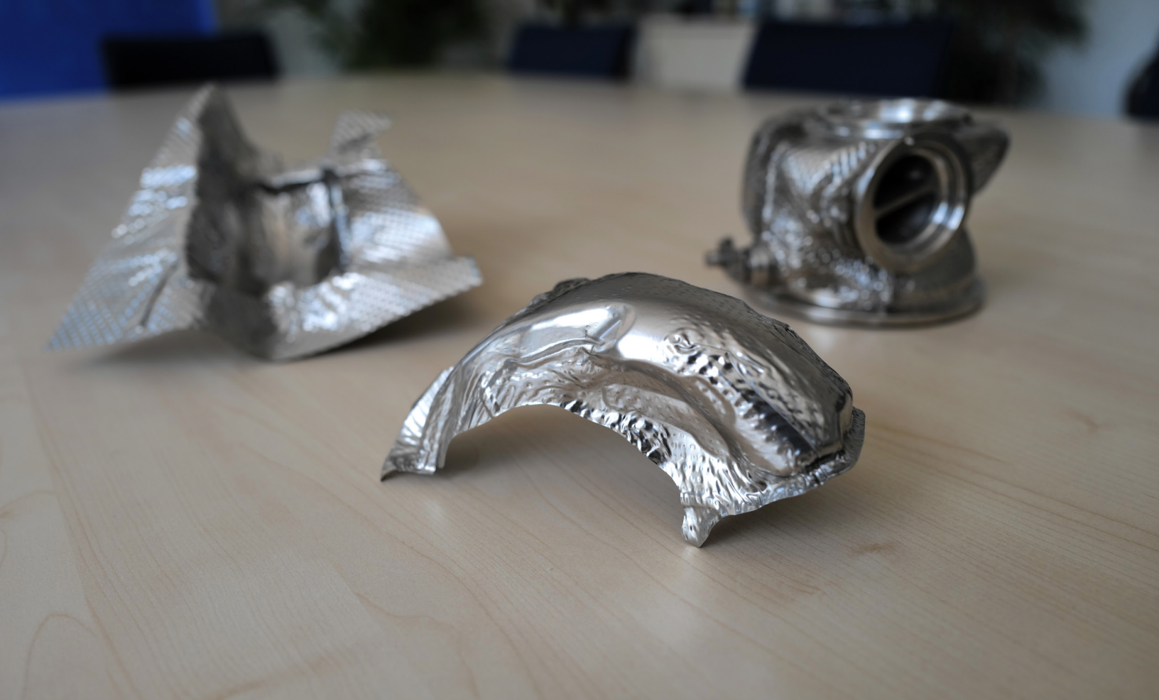
Half-shell for thermal insulation of turbochargers. (Pictures: © Kölle GmbH/ Stampack GmbH)
