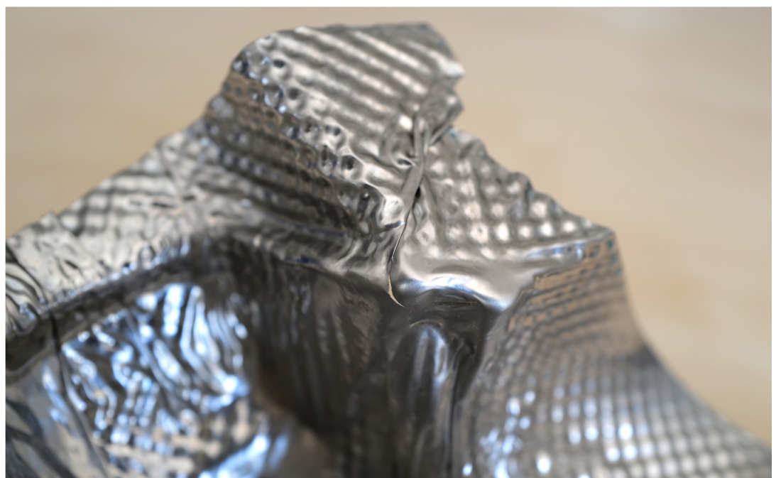
Cracked shell due to unfavorable folds.
